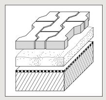
**Pavers:** minimal thickness 0.06m. **Isolating layer:** sand bed, 0.06m minimum.
