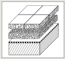
**Slabs:** precast concrete or hard stone (thickness  $\geq$  0.04m; length/ width from 0.25 to 0.50m) wide joints, 0.02m approximately, filled with mortars, or tight joints.
