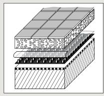
**Bedded or bonded floor covering:** in principle, not laid by the waterproofing contracting firm .
