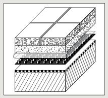
**Slabs:** precast concrete or hard stone (thickness  $\geq$  0.04m; length/width from 0.5 to 0.50m), joint between slabs 20mm approximately, filled with mortar.
