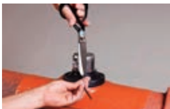
Cut off the the remaining part of the cable tie.
