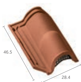
Ventilation tile 5.0 kg each - Ventilation section: 36 cm 2
