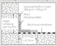
In some cases (see CCP), the use of Supracoating RLV enables the elimination of water drainage systems. Supracoating RLV withstands thermal shocks caused by asphalt casting.
