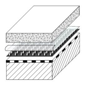
Mortar or concrete screed: Minimum thickness 0.04 m. Mixed with a water-reducing plasticizer.
