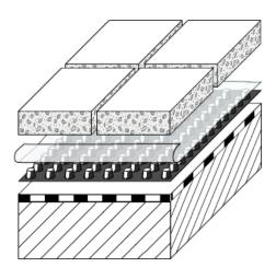
Precast concrete slabs: laid dry, joints dry Dimensions 0.40 to 0.60 m for walkways
