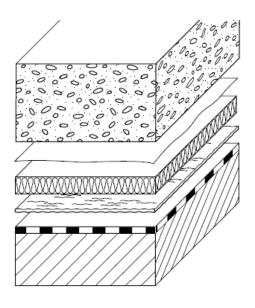
Reinforced concrete paving:
