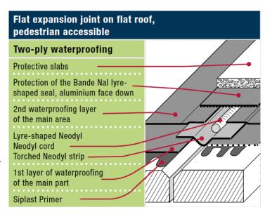
The Neodyl System is used for structural expansion joints on pedestrian accessible roofs, roof gardens and non-accessible exposed roofs. Suitable for all roof substrates.
