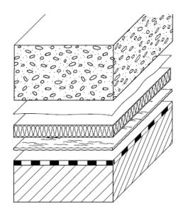
Reinforced concrete paving: Mixed with a water-reducing plasticizer Separation layer:
